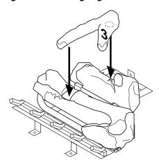
Figure 55 - Installing Log No. 3
